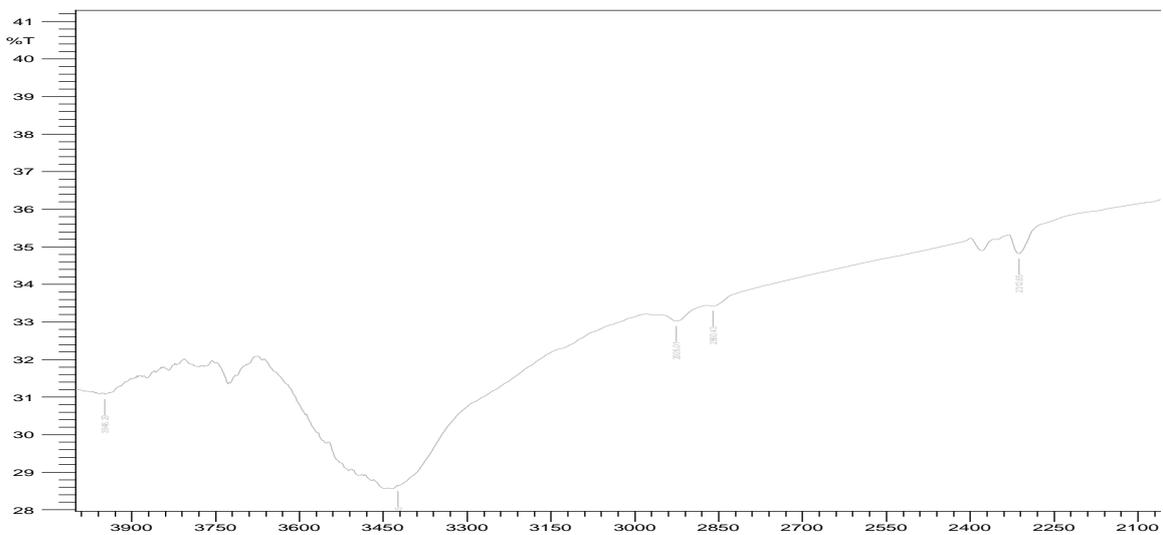
Fig. 6. FTIR spectra of silver nanoparticles recorded in the range of 2300-4000 cm<sup>-1</sup>
